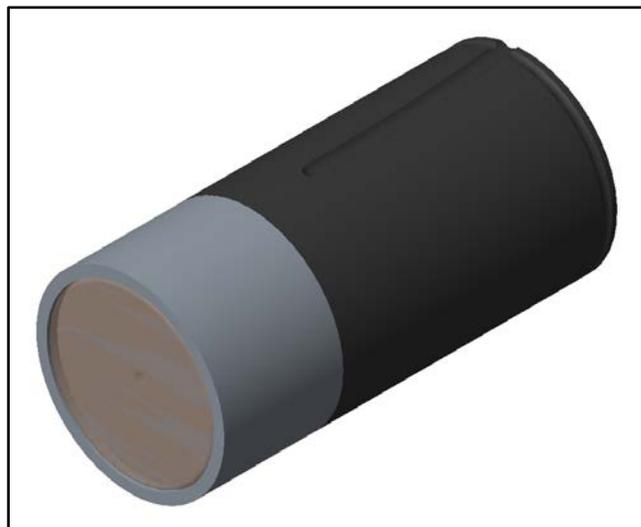
**Model of projectile showing slight helical groove, aluminum foam nose pad, and bonding adhesive**
