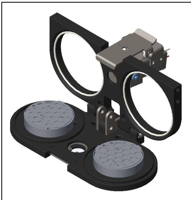
**Open barrel door assembly (inverted) showing the projectile adhesive heaters, latch, and laser**
