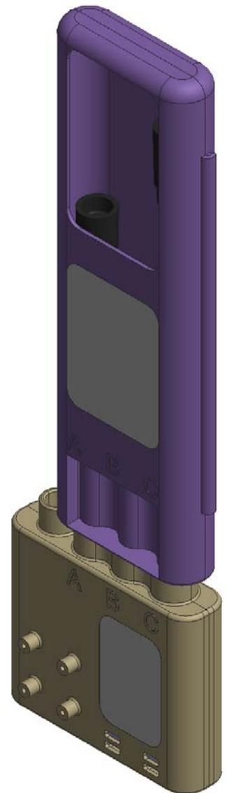
**Model of the swab carrier inserted into the test unit during test detection**
